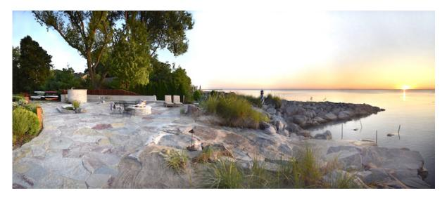
"Because of the water that will be pouring off these boats, we changed the pattern over the course of the patio," says Benz. "Around the patio, it's a crazy-quilt pattern with tight joints. With the boat storage, it's more loosely laid so the water can get out of the area."
