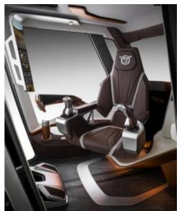
The ergonomic and comfortable seat features industry-first automatic pivoting functionality.
