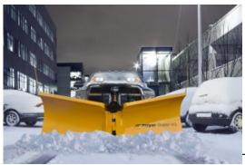
The Super-V3's Standard Operating System has a streamlined appearance with an encased power unit and patented cable management system for reliable service. The hydraulic system also features an adjustable drop speed to handle various plowing conditions and meet operator preferences. Additionally, an exclusive upper-sealed center deflector keeps snow and ice off the windshield. On the bottom is an integrated urethane center cutting edge that eliminates snow trails left by ordinary V-plows.
