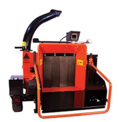
A triple-banded belt drive generates positive power, and a hydrostatic feed control provides the operator with infinite feed settings for all types and
