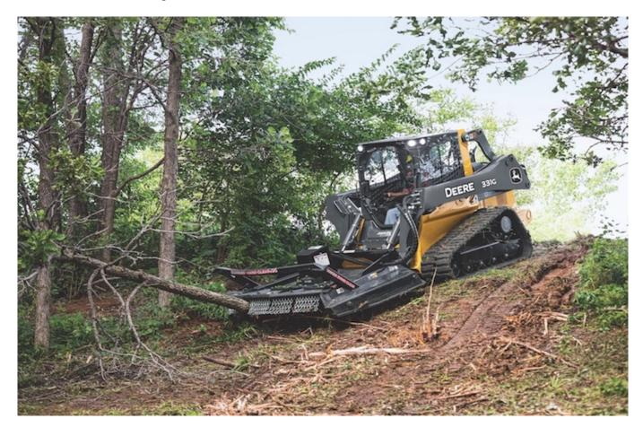
John Deere has updated its line of rotary cutters with the new RX72 and RX84 attachments. These new models are designed for heavy-duty vegetation management applications, including property maintenance and right-of-way clearing. The rotary cutter attachments are compatible on large-frame skid steer and compact track loaders, such as the 330G through the 333G, and they are equipped with high-flow hydraulics and a severe-duty door.
